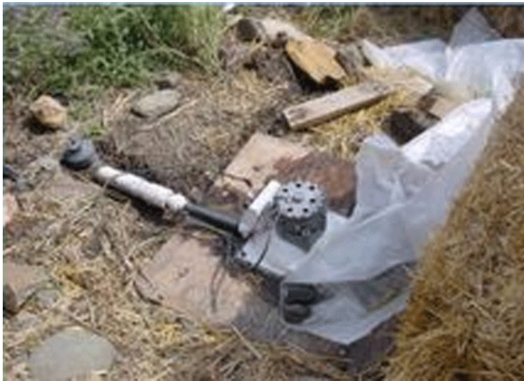
The hydropower unit, a wise use of the creek.
